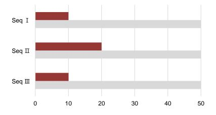
Foaming test : XTeer ATF Ⅲ reduces generation of foam.
